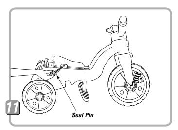
• While pushing down on the seat, insert the seat pin through the hole in the seat and into a seat mount adjustment hole.
